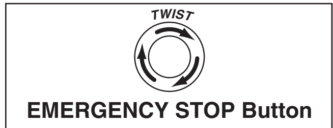
Figure 15. Resetting the EMERGENCY STOP switch.
